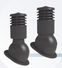
Insulated ventilation chimneys with diameters of 125 and 150 mm — the upper part of the chimney is insulated to prevent the decrease in the condensate temperature and to effectively extract the wet air outside. Insulated chimneys are used to ventilate rooms with increased humidity, such as kitchens, bathrooms and laundry/drying rooms. Using uninsulated chimneys for such rooms can result in condensation in the ventilation duct, which means that the condensate can return to the room.
